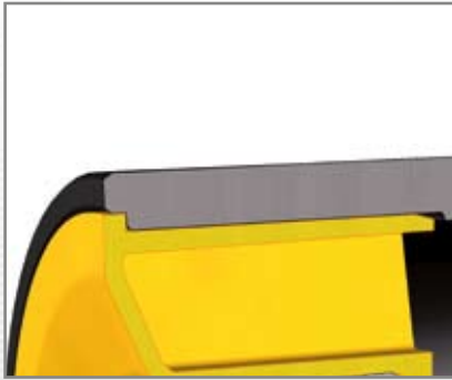
High Density Polyethylene (HDPE) tube, black colour, long fitting between the tube and the bearing housing
